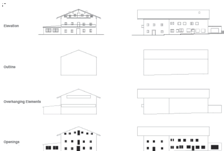
Fig. 34: AlpHouse pilot-building E. in Schleching, layers of facade, by TUM Landraum
